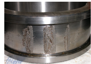
Damaged High - Speed Bearing
