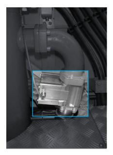
The sensor can then be wired from its standard M12 connector to an existing CMS system (if equipped) already provisioned for MetalSCAN, to an Ethernet network connection, or to an optional module for cellular connection. Simply follow the step-by-step installation instructions included with the MetalSCAN package.
