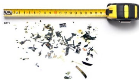
Metal Debris from B-Sump Screen
