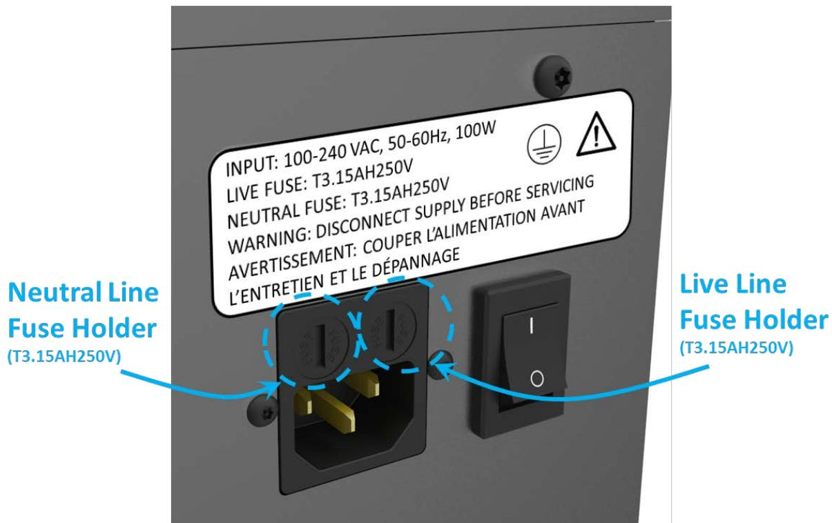
Figure 6-3: Power Entry Module and Main Power Switch
