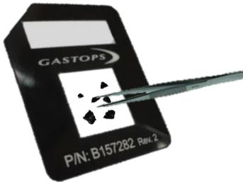
4. Re-apply the protective cover onto the Sample Patch window. This is to protect the sample prior to analysis.
