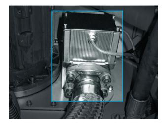
The sensor can then be wired from its standard M12 connector to the turbine controller input channels already provisioned for MetalSCAN, to an Ethernet network connection, or to an optional module for cellular connection. Simply follow the step-bystep installation instructions included with the MetalSCAN package.
